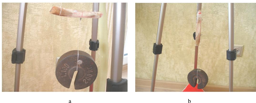
Fig. 5. Application of force with vertical (a - 1 kgf) and horizontal (b - 2 kgf) position of the rib.
